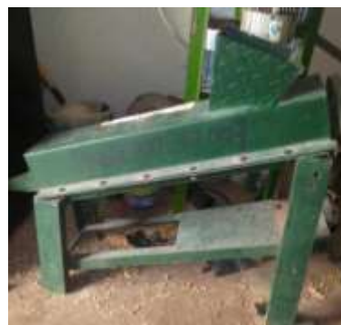
Figure4: Fabricated Maize-shelling machine
