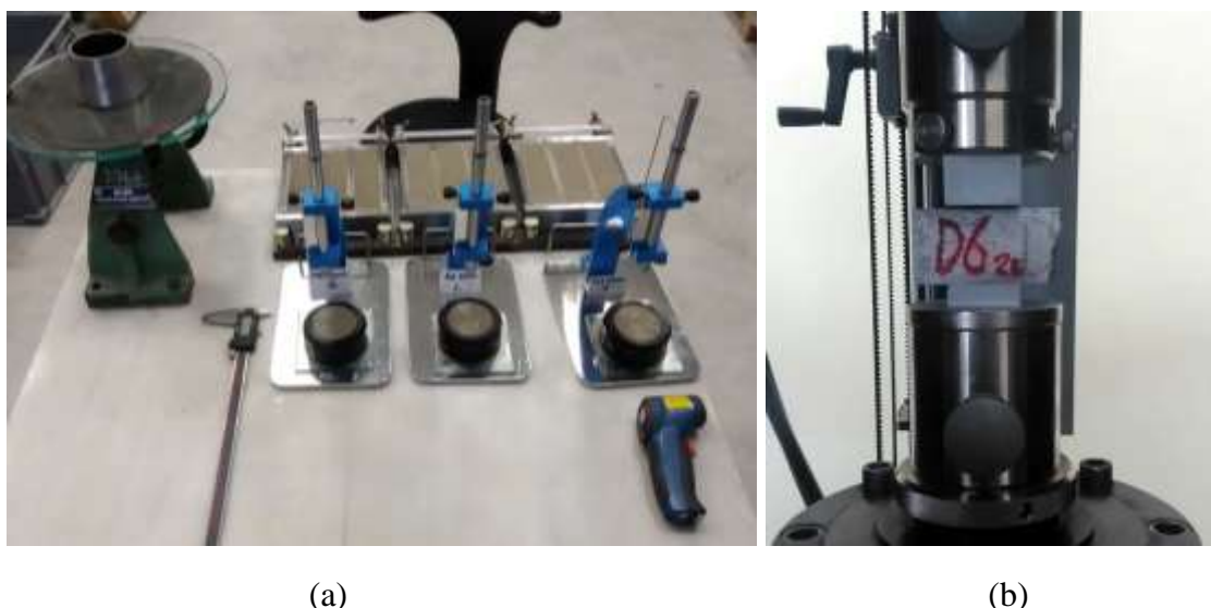
Figure 2. a) Flow table, vicat tests and casted specimens, b) Compressive tests.
